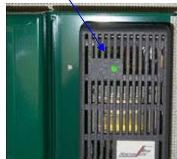
battery is totally charged when the control light goes out.
